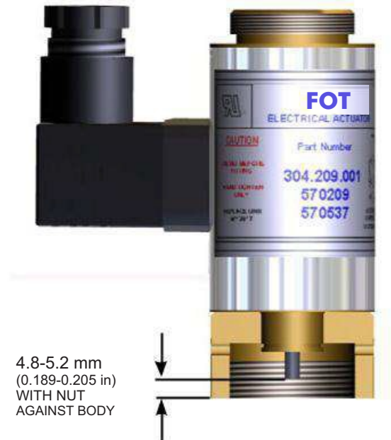
Actuator Non-Fire Position
