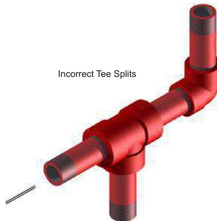
Side tee orientation "incorrect"
