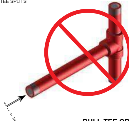
BULL TEE ORIENTATION "INCORRECT"
